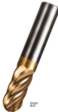
After reaching a tilt angle of at least 22°, then all six edges will at least be partially engaged.
