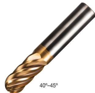
For maximum profiling performance, a tilt angle of 40°-45° will result in full engagement of all edges with a wide range of cutting depths.
